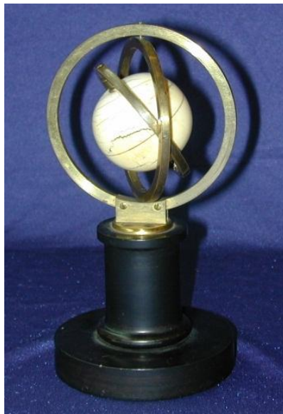
Figure 1: Machine of Bohnenberger, as described in original publication of 1817.
