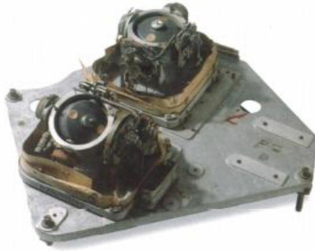
Figure 2: Gyros used for German V2 rockets during World War II.
