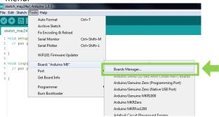
Install latest version of "Arduino SAMD Boards (32-Bits ARM Cortex M0+)"
