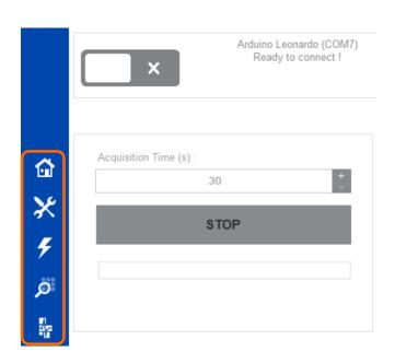
Once the Arduino board is detected by the software, you can click on the top left power ON/OFF button. The application will start and read the sensor information (serial number and type of sensor).
