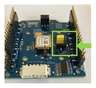
6. Plug the GYPRO® or AXO® Evaluation Board on the Arduino Board, using the 5 connectors supplied by Tronics. The correct position is to have the Arduino board on top (above the Evaluation board).
