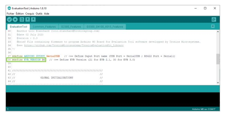
2. Upload the program: Simply click on the "Upload" button in the environment. Wait a few seconds, and you should see the RX and TX LEDs on the board flashing. If the upload is successful, the message "Done uploading." will appear in the status bar at the bottom of the window.
